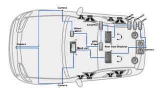
Fig 1 MOST ring topology. All devices see entire network traffic from every other devices
