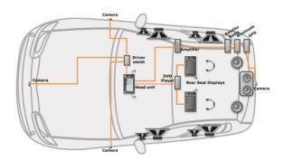
Fig 2 Possible AVB architecture. In this example, the camera signals from the front of the car only pass to the drives assistance module.
