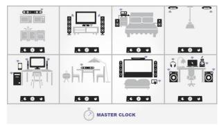
Because audio and video signals require many different clock rates, every AVB device in the network continues to generate audio and video timing signals using its own clock. The difference with AVB is that this clock will now be synchronized with the other AVB clocks on the network.
